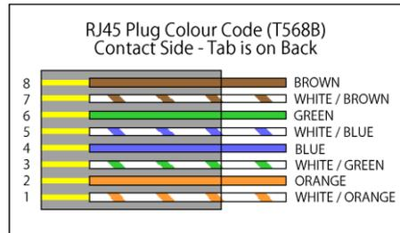
**IMPORTANT:** The signals used by this extender set will not pass through any Ethernet device. The Matrix and Receivers provided in this set will only work with the Xcalibur product range. Please make sure that the Cat6 cable uses 4 pairs of 23AWG solid copper wires. Do not use inferior copper clad cables as these exhibit high resistances.
