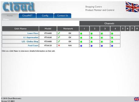
A green indicator in the **Channels** columns confirms that each channel of each amplifier is operating normally.
