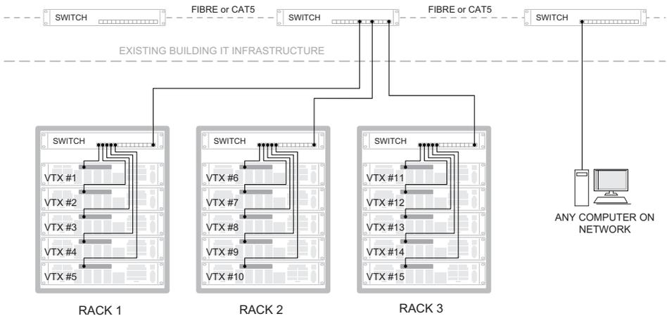
As many amplifiers and racks as required can be networked in this way, and these may, of course, be anywhere in the building. The only requirement is that each rack switch is connected to the same building network, so that all amplifiers in the system are accessible from a computer elsewhere on the network.
