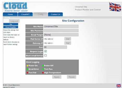
5. Enter a suitable name for the installation in the **Site Name** field (e.g., name of the customer and/or building or location, etc.)
