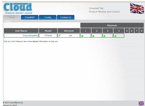
The amplifier type listed in the **Model** column should be that of the amplifier being addressed.
