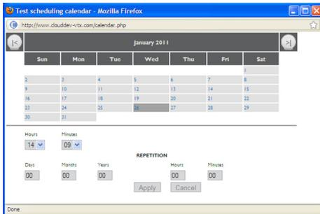
Select the date on which the next test is to be run by clicking on it. The months can be scrolled through with the '<' and '>' buttons at the top. Next select the time at which the test is to be run using the **Hours** and **Minutes** spin boxes.
