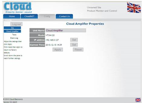
10. The first field, **Unit Name**, permits the amplifier itself to be named. This is extremely useful with large systems employing multiple amplifiers. Each amplifier will be referenced by the Unit Name on all the GUI pages thereafter. The name may, for example, be the area of the building where the speakers that the amplifier is driving are located. (The Unit Name may be up to 100 characters in length, but note it will be truncated to 16 characters for the amplifier button label.)
