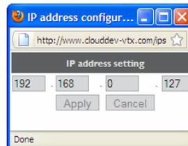
12. Enter the IP address for the amplifier in the four numeric fields and click **Apply**. We strongly recommend that you keep a careful record of all IP addresses used, and also write the address in the IP space on the VTX-WMI's rear panel (or print a label for this purpose).
