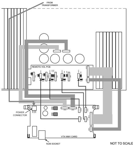
8. The VTX-WMI card can now be fitted in place; the two rear supports should engage with the edge of the heatsinks, and the RJ-45 Ethernet connector should protrude through the rear panel slot. The two previously empty holes in the amplifier rear panel should align with the tapped holes in the card's rear brackets; secure the card using the two screws supplied.
