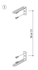
Fix mounting brackets on solid surface (recomended distance between brackets center holes 56 mm for COM 40 and 31 mm for COM 20)
