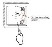
2. Fix the loudspeaker cabinet with screws.
