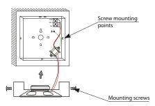
4. Select desired power and attach front panel to the cabinet. Connect loudspeaker to the transformer.
