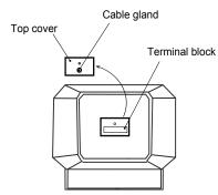
2. Remove top cover, insert the cable in to the cable gland and connect the cable to terminal block.
